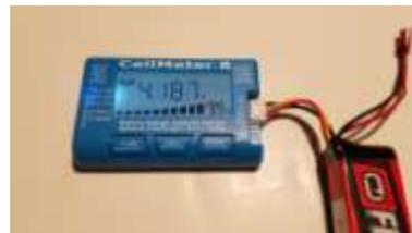
Here is a very nice new battery checker above right for outdoor flyers; it's about \$12 from Amazon, it will check up to 8 cell LiPo's and also has a servo tester built in. RC Digital Battery Capacity Checker Tester, Cell Meter 8 LiPo Battery Discharger Balancer, RC Servo Tester LCD Backlight Updated Version
